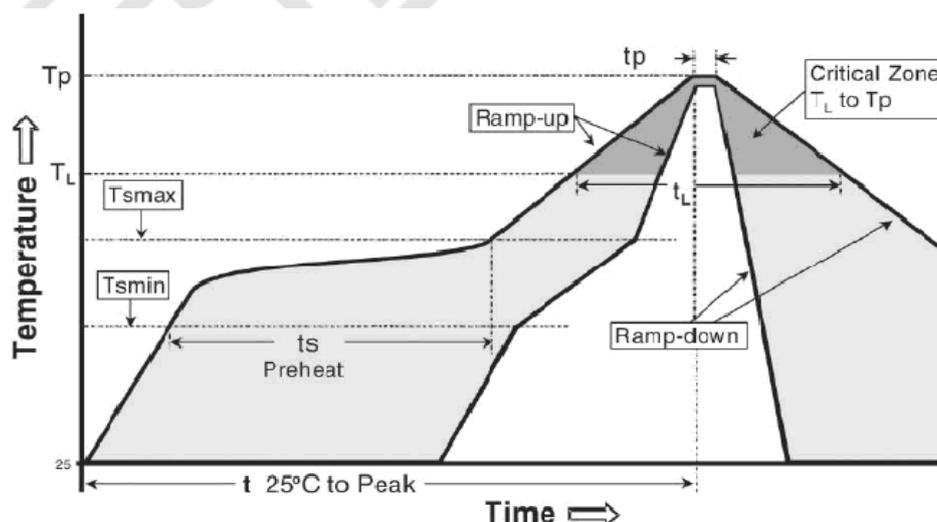
焊接图-1 Classification Reflow Profile
